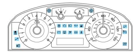
Warning lights and gauges can alert you to a vehicle condition that may become serious enough to cause extensive repairs. A warning light may illuminate when a problem exists with one of your vehicle's functions. Many lights will illuminate when you start your vehicle to make sure the 12
